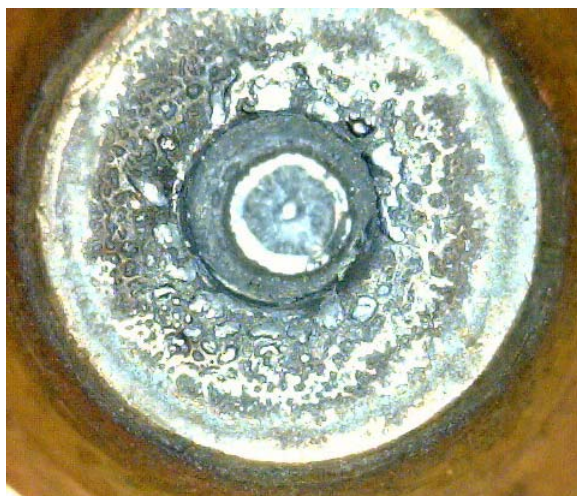
Figure 60 – Non-symmetrical, rough-edged pit and rough-surfaced electrode face
