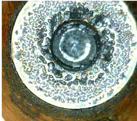
Figure 59 – Wide electrode pit that extends beyond the hafnium
